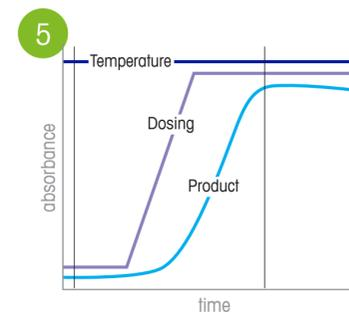
**The Chemistry:** By studying how chemistry changes as process conditions are varied, scientists can determine which process parameters will deliver optimized reactions
