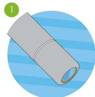
**The Sensor:** ReactIR™ Comp™ sampling technology places the sensor directly into the reaction for continuous, real-time monitoring
