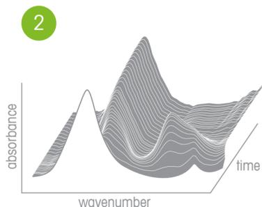
**The Measurement:** Spectra are continuously collected and presented in a water fall plot - absorbance vs. wavenumber vs. time
