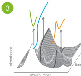
**The Peaks:** Use iC IR™ software to identify isolated peaks that change over time. 'Profiling' those peaks shows how they change over time. Consider using the Find Trends function.
