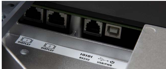
Figure 5-14: Display Connector Sockets
