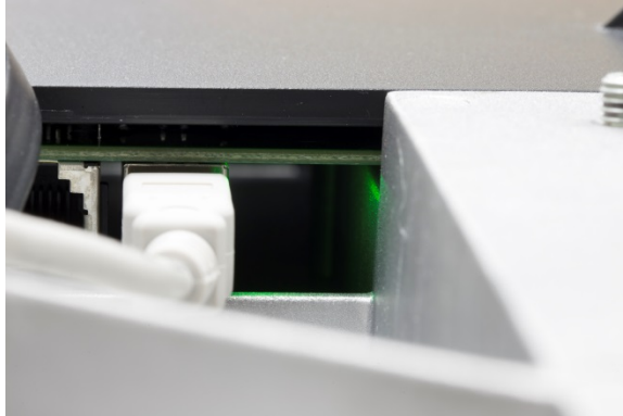
Figure 5-1: Green PCB Status Light Illuminated
