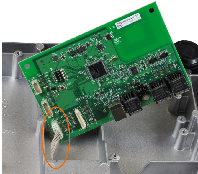
Figure 5-11: Load Cell Harness Connected to PCB
