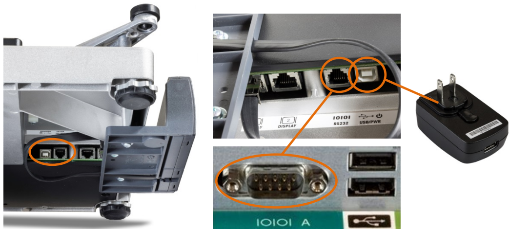
Figure 2-5: Serial Connections, Scale(left, top) and PC (bottom center); Power Supply (right)
